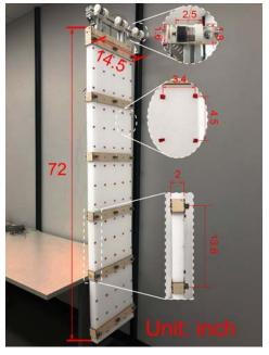
Fig. 4. Dimensions of the built prototype.
